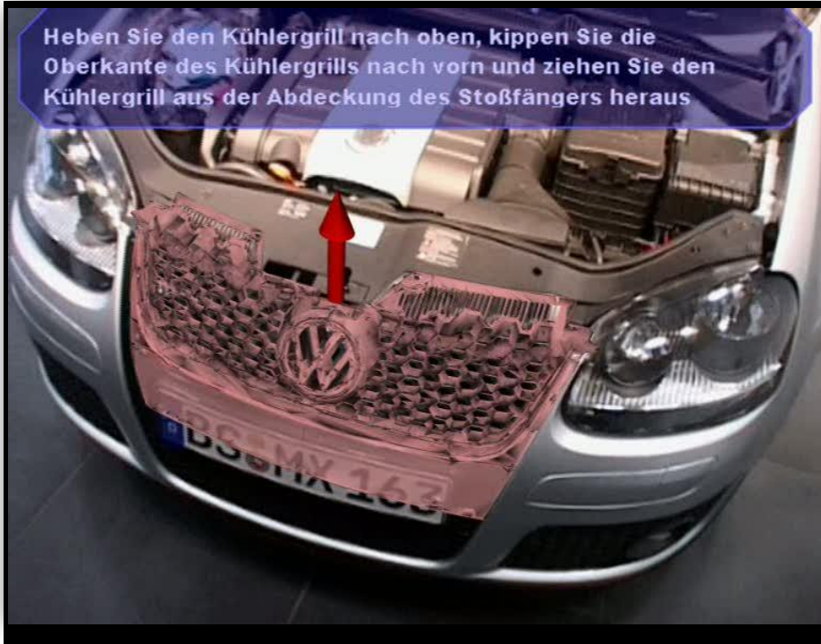
3D task overlay for car maintenance
